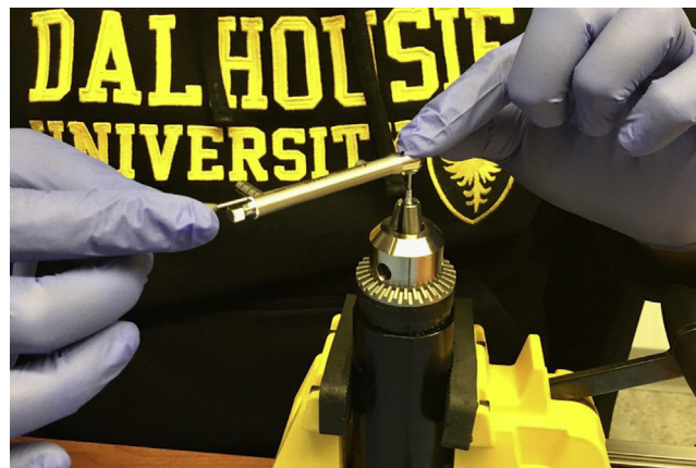
Figure 3. Mechanical torque limiting device used to tighten abutment screw while second operator read torque applied.
