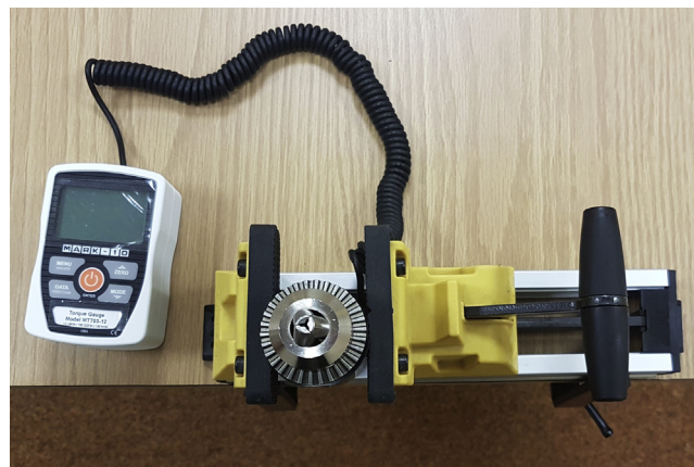
Figure 1. Digital torque gauge secured to table by using precision vise.
