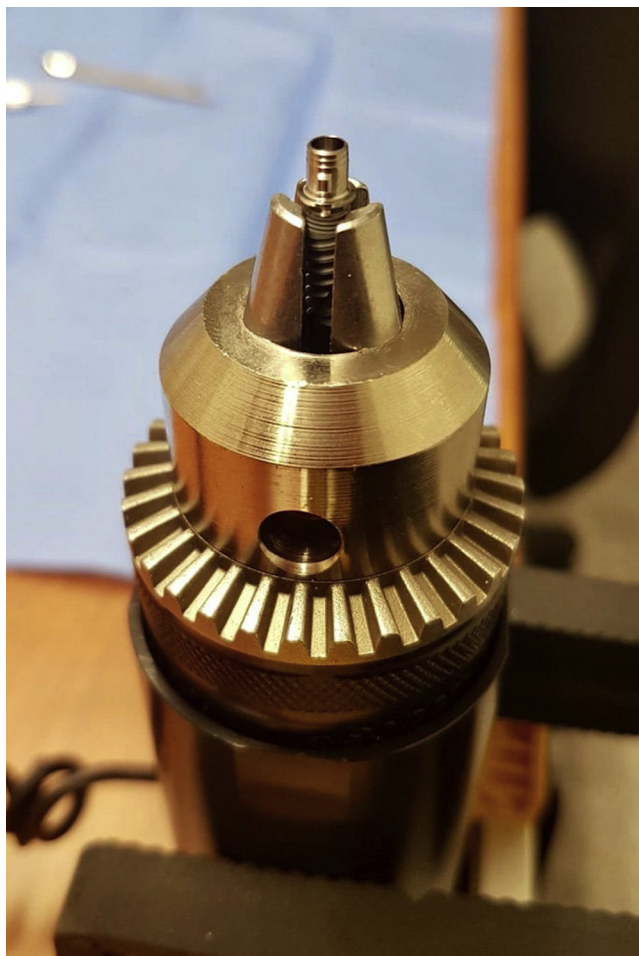
Figure 2. Implant and universal base abutment secured in 3-jaw chuck of digital torque gauge.
